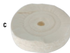
C BUFFING WHEEL, SISAL Approx. 70 layers of especially evenly woven sisal, double sewn, for fine polishing. Fits mandrel for felt wheel (No. 705491). Centre hole 20 mm Disc Ø 150 mm Width 20 mm No. 705496
