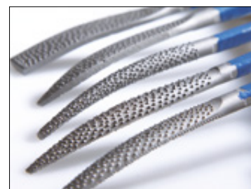
A HERDIM® RIFFLERS, 8-PIECE SET Crafted and hardened with great care by master craftspeople. For shaping convex and concave surfaces. The teeth are cut on both sides, the ends bent in opposite directions. Square mid-section. Comes in a leather roll. Flat, warding, trapezoid, square, three-square, half-round, crossing, round. Cut 4 Cut length 55 mm Overall length 185 mm No. 704599
