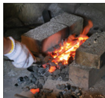
Forging a hoe head
