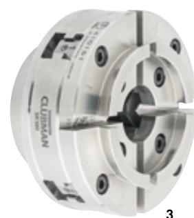
3 SK100, with Type C Jaws Model M33 x 3.5 DIN 800 Ø 100 mm External chucking 52-66 mm Internal chucking 66-80 mm 1.6 kg (solo) No. 702240
