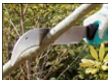
F SAJI NATA This archaic-looking cleaver with a single bevel is ideal for cutting flush to the trunk. Takeshi Saji welds the shock-absorbing part of the double-layered blade to a cutting layer of White Paper Steel in the fire. The result is a blade that is both resistant and has good edge retention. The blade is securely anchored in the oak handle by a ferrule. Scabbard made of magnolia wood with leather mounts; can be worn on the belt. Head weight 330 g Blade length 195 mm Overall length 360 mm No. 710864
