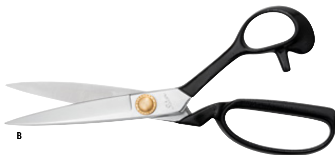
B PROFESSIONAL TAILOR'S SCISSORS Professional tailor's scissors with a double-layered blade. Crafted from White Paper Steel, the high purity and high carbon content (1.2 %) of the cutting edge guarantee superb sharpness and durability. The edge layer is not rustproof; chromed to protect against rust, brass screw. Hardness 60 HRC, not rustproof.
