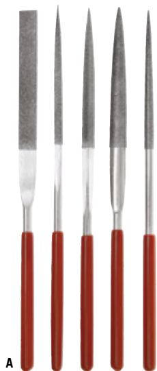
A DIAMOND NEEDLE FILES, POLYCRYSTALLINE, 5-PIECE SET Flat 9 x 2.3 mm, half-round 9 x 3 mm, square 4.5 mm, three-square 6 mm, round 5 mm. Grit D107 **. Coating length 70 mm Overall length 180 mm No. 711045
