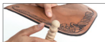
E EDGE SLICKER, 4 WIDTHS For burnishing leather edges after skiving with an edge beveller or an edge trimming plane. Use the four U-shaped profiles to slick leather up to 10 mm thick. The edge slicker is ideal for hard-to-reach, tight spaces, perforations and narrow curves.
