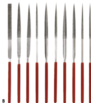
B DIAMOND NEEDLE FILES, POLYCRYSTALLINE, 10-PIECE SET Flat 6 x 1.5 mm, half-round 5 x 2 mm, square 2.5 mm, three-square 3.5 mm, round 3 mm, warding 5 x 1.5 mm, knife-shaped 5 x 1.5 mm, barrette 5 x 2 mm, crossing 5 x 2 mm, crossing 3.5 x 2.5 mm. Grit D107 **. Coating length 50 mm Overall length 180 mm No. 711044
