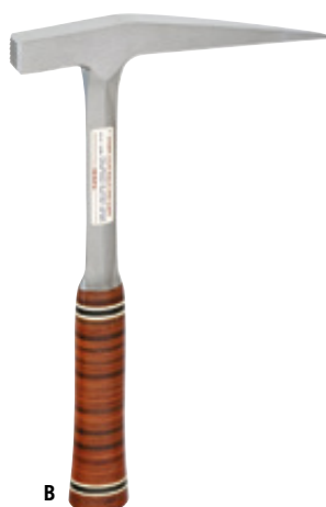
B ESTWING® ROCK PICK A rock pick is a combination of a hammer and a pick. The long, hardened, pointed tip allows stones to be struck with extreme accuracy, and thus split with precision. The end of the handle is riveted Head weight 390 g Overall length 320 mm No. 705697
