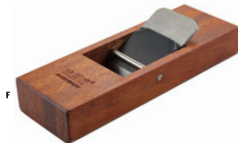
F SMOOTHING PLANE, BEVEL UP This Chinese »bevel up« plane features an adjustable cutting angle by changing the micro bevel. Indonesian redwood body. Blade angle 25°, bevel angle 20°. This results in a cutting angle of 45°. Comes with HSS blade and chip-
