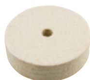
A COTTON POLISHING DISC White cotton disc, 6-fold stitched. For mirror polishing with polishing pastes. For arbors with Ø 10 mm. Fits holding arbor No. 728800. Bore 10 mm Disc diameter 75 mm Disc width 10 mm No. 728818
