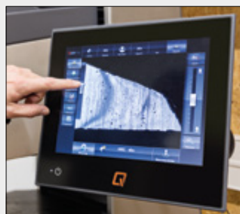
Tooth checking by microscope
