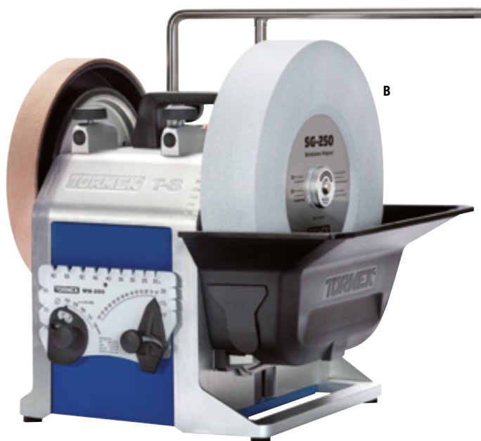
B TORMEK® T-8 ORIGINAL »Tormek Original« sharpening wheel (SG-250), aluminium oxide, Ø 250 x 50 mm, grit 220; leather honing wheel, Ø 215 x 30 mm; universal support, finely adjustable (can be used horizontally or vertically). 230 V, 200 W, 90 rpm, torque 14.7 Nm, 14.8 kg.
