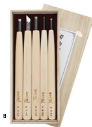
B CARVING KNIVES, 5-PIECE SET Light as a feather and razor-sharp, traditional Japanese tools for woodcuts, masks and reliefs. Thin, double-layered blades, White Paper Steel (63 HRC), sharpened ready-to-use. Magnolia wood handles. Blade thickness approx. 2 mm. Straight chisel 6 mm; skew chisel 9 mm; gouge sweep 8 / 4.5 mm; gouge sweep 9 / 9 mm; V-tool 4.5 mm. 5-piece set, comes in kiri wood box. Blade thickness 2 mm. Blade length 25-30 mm. Overall length 200-210 mm No. 710753
