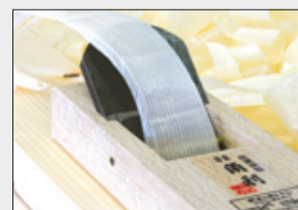
C CHAMFER PLANE With removable fence for 30°, 45° and 60° bevels. Carbon steel blade, approx. 62 HRC. Screw chipbreaker, Japanese white oak body. Blade width 20 mm Blade thickness 3.5 mm Overall length 150 mm 290 g No. 717033
