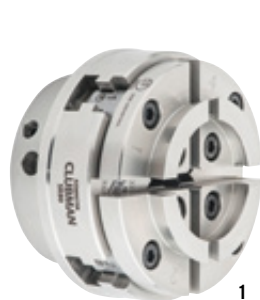
1 SK80, with Type C80 Jaws Model 1 inch x 8 tpi Ø 80 mm External chucking 34-68 mm Internal chucking 51-86 mm 1.3 kg No. 702274
