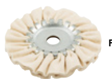
F FLANNEL POLISHING DISC Folded flannel, untreated, on sheet metal ring. For high gloss polishing with polishing pastes. Pleated rings show less wear and dust when roughened.
