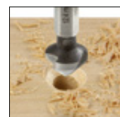
D 90° COUNTERSINKS WITH BIT HOLDER, 7-PIECE SET These HSS countersinks with three blades are suited for steel as well as light metal, for plastic as well as wood. The hexagonal shaft allows safe clamping without slippage and also insertion into quick-change bit holders. Comes in metal case (Ø 6.3 / 8.3 / 10.4 / 12.4 / 16.5 / 20.5 mm), with bit holder. No. 707469
