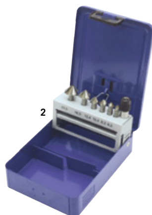
D 90° COUNTERSINKS WITH BIT HOLDER, 7-PIECE SET These HSS countersinks with three blades are suited for steel as well as light metal, for plastic as well as wood. The hexagonal shaft allows safe clamping without slippage and also insertion into quick-change bit holders. Comes in metal case (Ø 6.3 / 8.3 / 10.4 / 12.4 / 16.5 / 20.5 mm), with bit holder. No. 707469
