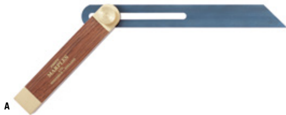
A ENGLISH SLIDING BEVEL, WALNUT Stock made of walnut with brass fittings. Angles are fixed through an adjustment screw, which is not in the way like a lever when marking or transferring angles.
