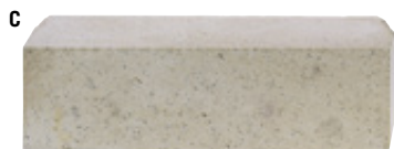
C JAPANESE NATURAL STONE »BINSUI« Medium-grit lime sandstone from the Kumamoto region for general sharpening. Readily absorbs water, cuts well and easily produces a fine slurry. Grit 800-1200 220 x 60 x 62 mm No. 711518
