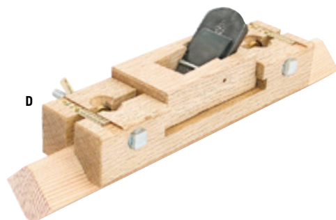
D CHAMFER PLANE, SKEWED For 45° bevels. The bevel width can be adjusted (0-16 mm). The chipbreaker and the slightly angled blade (skewed cut) allow it to be used even with random grain direction. Japanese white oak body.
