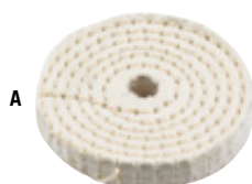
A COTTON POLISHING DISC White cotton disc, 6-fold stitched. For mirror polishing with polishing pastes. For arbors with Ø 10 mm. Fits holding arbor No. 728800. Bore 10 mm Disc diameter 75 mm Disc width 10 mm No. 728818
