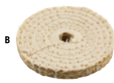
B SISAL DISC Untreated sisal disc, sewn in place. For pre-polishing all kinds of metal, even those with rough surfaces. Will result in a matt surface when used with coarse polishing paste. Fits holding arbor No. 728800. Bore 10 mm Disc diameter 75 mm Disc width 10 mm No. 728817
