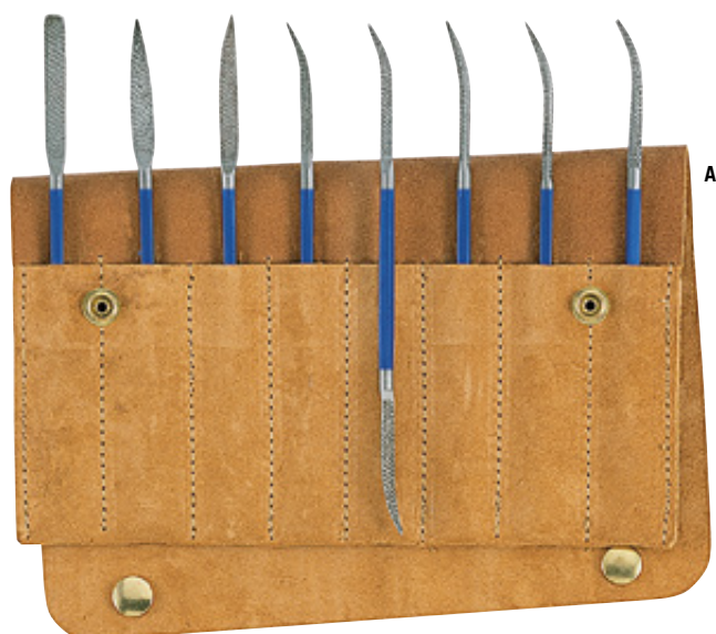
A HERDIM® RIFFLERS, 8-PIECE SET Crafted and hardened with great care by master craftspeople. For shaping convex and concave surfaces. The teeth are cut on both sides, the ends bent in opposite directions. Square mid-section. Comes in a leather roll. Flat, warding, trapezoid, square, three-square, half-round, crossing, round. Cut 4 Cut length 55 mm Overall length 185 mm No. 704599
