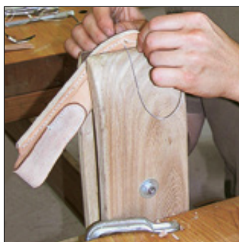
A DICTUM® STITCHING PONYS Solid wood stitching pony in an elegant design with integrated aluminium hinge. Practical base plate for clamping on table tops or worktops. Max. mouth opening 45 mm, mouth width 90 mm, mouth depth 150 mm, arm length 270 mm. Overall length 350 mm 1.2 kg No. 708171
