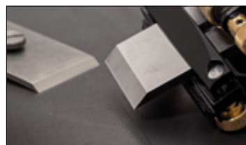
Ready-to-use grind with micro bevel
