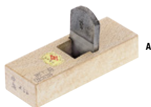
A SCRAPING PLANE Vertical blade. For trueing the soles of Japanese planes, working very hard woods and thin pieces. Plane across or diagonal to the grain. Japanese white oak body. Blade width 42 mm Blade thickness 6 mm Overall length 155 mm 400 g No. 717015
