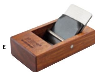
E BLOCK PLANE Compact, rectangular-shaped body, made of Indonesian redwood. HSS blade with chipbreaker, no wedge. Also ideal when working with leather, e.g. to sharpen leather edges. Blade width 44 mm Blade thickness 3 mm Overall length 105 mm 210 g No. 703276 Repl. Blade No. 702957
