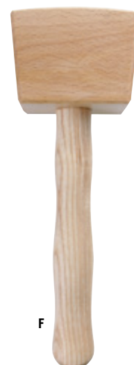
F HATTORI® SQUARE Mallet Simple square-headed mallet offering good value for money. For driving chisels, sculptor's gouges and for all tasks that require a wide striking face. With impact-resistant red beech head with bevelled edges, and ash handle wedged to the head. The oval shape of the handle makes it easy to align the striking face with the workpiece or tool. Head width 65 mm Overall length 305 mm 440 g No. 730047
