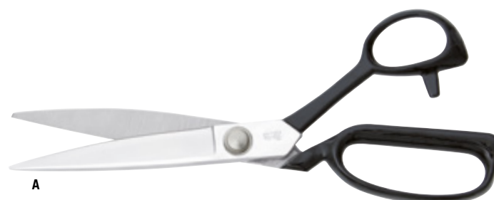
A TAILOR'S SCISSORS Tailor's scissors made of SK5 carbon steel (C 0.85 %), chromed to protect against rust. Black painted handles. Hardness 59 HRC.
