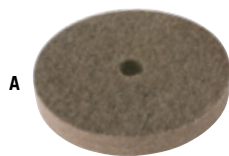
A FELT POLISHING WHEEL, MIXED WOOL FELT, STRAIGHT Smoother felt, takes more polishing paste, enables more intense abrasion. Fits mandrel for felt wheel (No. 705491). Centre hole 20 mm Disc Ø 150 mm Width 20 mm No. 705493
