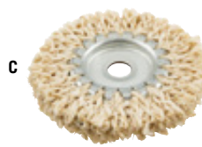
C SISAL CORD DISC Untreated sisal cords in radial direction on sheet metal ring. For pre-polishing, especially of profiled parts. After longer use, the sisal cords become more flexible. For use with polishing paste. Fits holding arbor No. 728800. Bore 10 mm Disc diameter 75 mm Disc width 10 mm No. 728816
