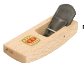
B COMPASS PLANE The sole is curved along its length and width, making it perfect for shaping seat bottoms, bowls, stringed instrument bodies etc. Japanese white oak body. Blade width 36 mm Blade thickness 7 mm Overall length 155 mm 340 g No. 717020
