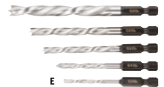
E FISCH® BIT WOOD TWIST DRILLS PROFESSIONAL, 5-PIECE SET High-quality HSS wood twist drills with hexagonal shaft for quick change of bits. The hexagonal design prevents the shaft from slipping in the case of impact loads, e.g. when drilling into knots.
