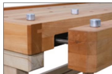
Worktop secured through breadboard end
