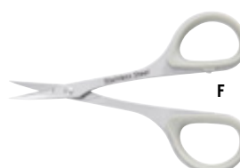
F THREAD TRIMMER Small thread trimmer with slightly curved blades. Lies firmly in the hand thanks to rubberised finger rests. Hardness 52 HRC, rustproof. Overall length 90 mm Blade length 20 mm 15 g No. 718372
