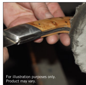
C BUFFING WHEEL, SISAL Approx. 70 layers of especially evenly woven sisal, double sewn, for fine polishing. Fits mandrel for felt wheel (No. 705491). Centre hole 20 mm Disc Ø 150 mm Width 20 mm No. 705496
