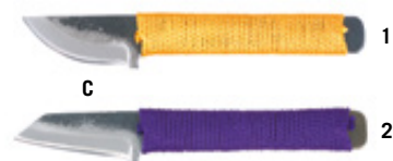
C CARVING KNIFE WITH CORD HANDLE Similar to the handles of Samurai swords, the handle of this Japanese carving knife is bound with silk cord. Slip-proof in the hand, it can be precisely guided, even with increased application of force. Triple-layered blade, core layer of Blue Paper Steel, hand guard, double bevel. Blade length 55 mm. Overall length 160 mm. Blade 1 curved No. 710747 2 straight No. 710749
