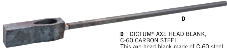
A WHITE PAPER STEEL FROM JAPAN The finest grain: Non-alloy Japanese carbon steel, finest martensitic structure. Extremely sharp, close to sword steel. With heat treatment instructions. 480 x 30 x 4.5 mm No. 719620
