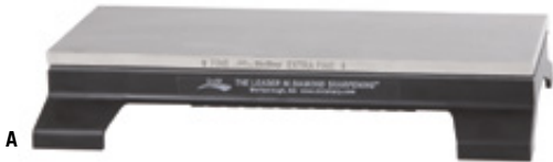
A DMT® DIA-SHARP® BENCH STONE WITH MAGNABASE Combination sharpening stone with continuous diamond coating on both sides on a solid steel base plate. The large sharpening surface is ideal for sharpening long knives and wide cutting edges on tools such as plane blades or drawknives. The torsion-re-
