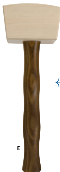
E DICTUM® SQUARE MALLETS These mallets are ideal for both assembly work and driving chisels. The hard, single-piece head of domestic white beech has a trapezoid shape for precise, ergonomic strokes. All edges are slightly bevelled to prevent damage to the workpiece. The smoked robinia handle has a double curve to perfectly fit the shape of the hand and is securely wedged to the head.
