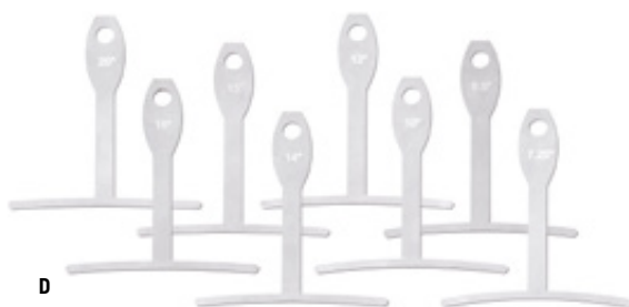
D HERDIM® UNDERSTRING RADIUS GAUGES, GUITAR, 8-PIECE SET Indispensable when setting and adjusting the magnets of the pickups. The gauge, only 3 mm high at the measuring base, can be slipped under the strings without their removal. The spokes have identical radius on the top and bottom, so the magnets can be easily adjusted according to the radius of the string pattern. Thickness 1 mm Radius 7.25", 9.5", 10", 12", 14", 15", 16", 20" Stainless steel No. 717089
