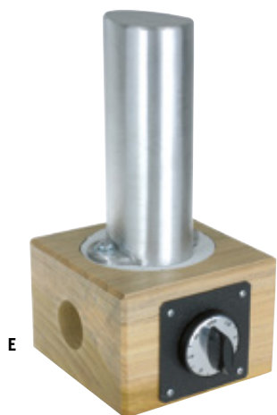
E UNIVERSAL BENDING IRON For violin, viola, cello, gamba and guitar. Cast aluminium body mounted on a wooden base with asbestos-free insulation. Can be used in a vertical or horizontal position. Thermostat control. 230 V, 200 W, Ø 50 x 80 mm, 1.8 kg. Working height 160 mm No. 703920
