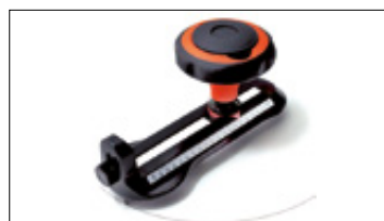
J HOLE CUTTER WITH KNOB HANDLE For guitar sound holes and rosette inlays. Centering tip, incl. four resharpenable blades in receptacle (knob handle), aluminium body with scale, knob handle with quick-adjustment mechanism. Ø 40-210 mm No. 716163 10 Repl. Blades No. 716169
