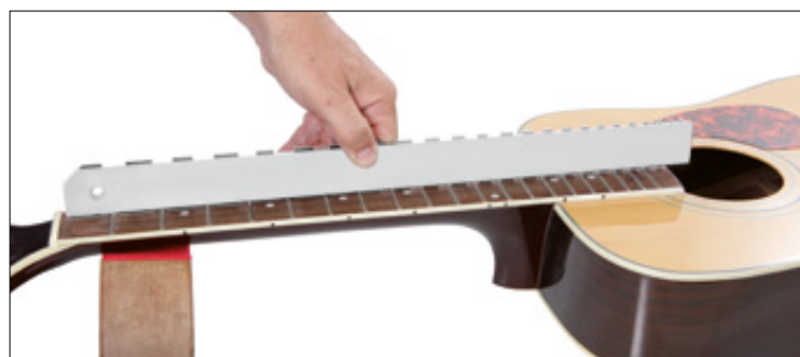
G FRETBOARD STRAIGHT EDGE, NOTCHED, GUITAR Steel ruler with precisely milled and sanded notched ruler edge for guitar fretboard straightness detection. Long and short scale notch pattern covers majority of fretting patterns. Instrument Guitar Thickness 5 mm Length 475 mm Steel No. 707014
