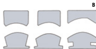
B HERDIM® PROFILE PATTERNS, 6-PIECE SET Precision patterns for shaping bridges and fingerboards. The tapered spurs at the base of the bridge patterns are for gauging the string height. 6-piece set for violin, viola and cello made of stainless steel. Sizes according to Hans Weisshaar. Thickness 0.5 mm No. 739400
