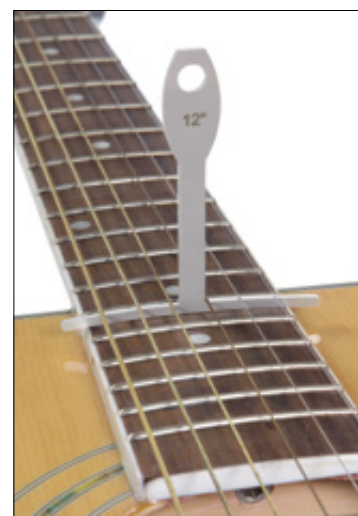
D HERDIM® UNDERSTRING RADIUS GAUGES, GUITAR, 8-PIECE SET Indispensable when setting and adjusting the magnets of the pickups. The gauge, only 3 mm high at the measuring base, can be slipped under the strings without their removal. The spokes have identical radius on the top and bottom, so the magnets can be easily adjusted according to the radius of the string pattern. Thickness 1 mm Radius 7.25", 9.5", 10", 12", 14", 15", 16", 20" Stainless steel No. 717089
