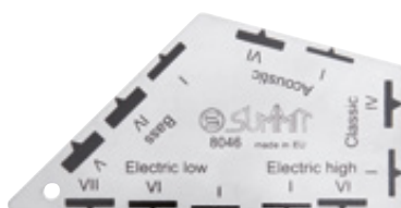
C SUMMIT® FRET ROCKER, GUITAR Fret rocker tool is traditionally used for pin-pointing of outstanding frets, which might cause fret-buzz. The tool has four different, precision ground edges, which can work on all fretted instrument fretboards. Thickness 1.5 mm Stainless steel No. 707049
