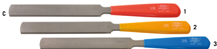
C UO-CHIKYU FRET FILES Concave, curved precision file for rounding fret crowns off after trueing. Total length 200 mm Sweep length 100 mm
