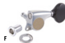
F NO. SGL510Z-BL5 Gotoh's top of the line tuner series. For acoustic guitar. X-Chrome-Finish, gear ratio 1:21, diameter 10 mm. Set: 3 x right, 3 x left. Artificial ebony buttons. Set No. 582216
