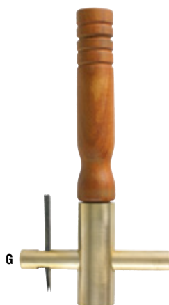
G MACH ONE PURFLING CUTTER Comfortable tool for cutting the purfling grooves on stringed instruments. The blade is guided smoothly by the precision mechanism. Fruit wood handle, brass body. Incl. 2 blades. Length 140 mm, diameter 18 mm No. 702544 2 Repl. Blades No. 702545
