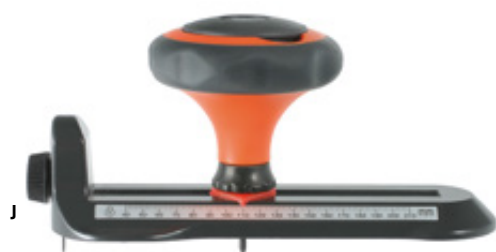
J HOLE CUTTER WITH KNOB HANDLE For guitar sound holes and rosette inlays. Centering tip, incl. four resharpenable blades in receptacle (knob handle), aluminium body with scale, knob handle with quick-adjustment mechanism. Ø 40-210 mm No. 716163 10 Repl. Blades No. 716169
