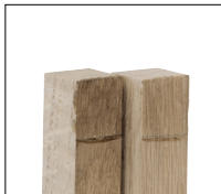
Missing bond between wood and glue – a clear adhesive failure.
