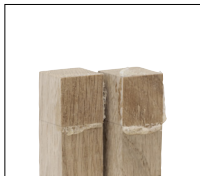
A break in the glue line is also a cohesive failure.
