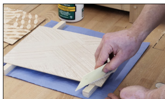
Step 3: The surface is evenly covered and ready to lay the veneers.
