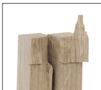
Fracture in the wood – a clear cohesive failure.
