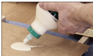
Step 1: Apply the glue to the middle of the surface.
