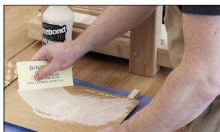
Step 2: Spread the glue from the centre outwards.
